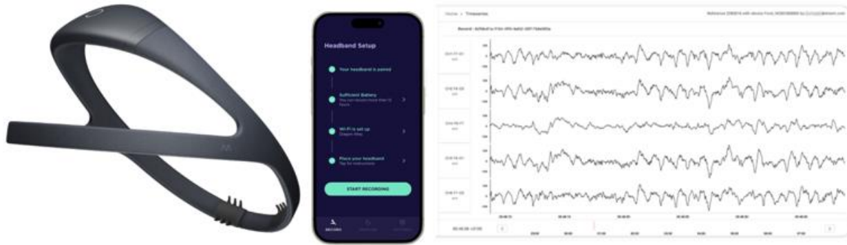
FIGURE 1: WAVEBAND HEADBAND, THE BEACON PAL APP, AN EDF OUTPUT OF THE DEVICE (LEFT TO RIGHT)
