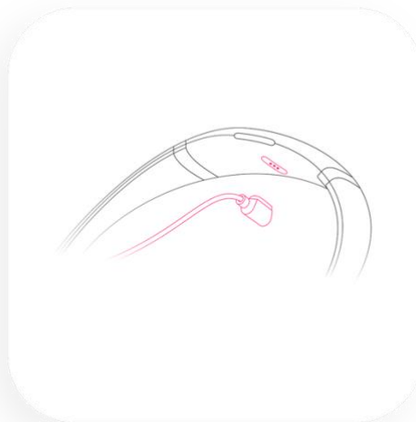
FIGURE 12: PLUGGING THE MAGNETIC CABLE
